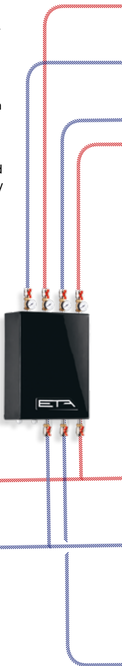
The ETA mixing circuit module for two heating circuits saves a lot of time and money during installation, as no sensor lines, pumps or mixer cables have to be installed.
