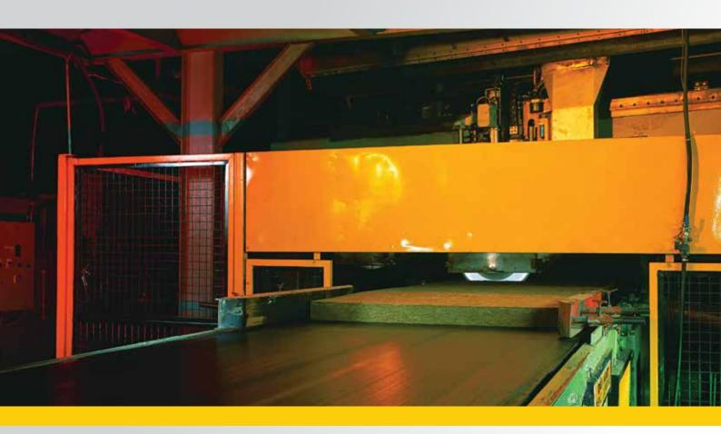
Stone wool is made from, an inorganic raw material, which is obtained domestically. It is produced through heating row material at 1350°C - 1400°C and transforming it into fibres. It can be manufactured in the forms of blanket, board, pipe or loose in different size and with different technical properties, with different facing materials according to the intented use and the place of use. It is used for thermal insulation, sound insulation, acoustic comfort as well as fire safety.
